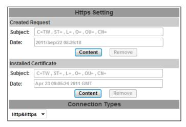
Https setting: Before setting new request, please remove old secure identification identification at Http connection type.
