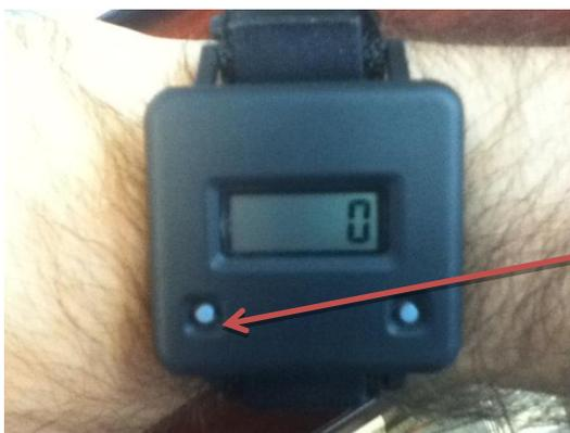
This is what the display should look like after you have activated the bite counter (the number of bites or calories will increment with each bite or the device will simply display the word "on").
