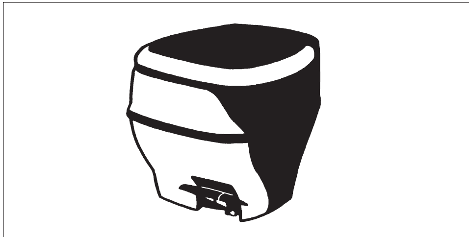
FIGURE 12 TYPICAL FOOT PEDAL MARINE-TYPE TOILET
