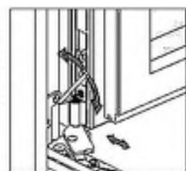
i) gasket pressure adjustment (concealed hardware)
