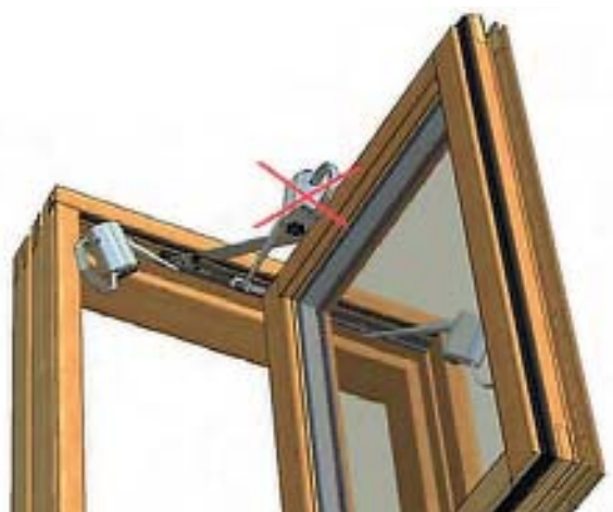
Figure 7.4. Lubricating a side projecting gearing
