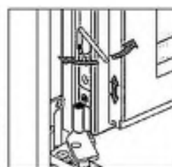
h) Vertical sash adjustment (concealed hardware)
