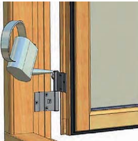
Figure 7.1. Lubricating a butt hinge
