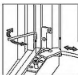
g) Horizontal sash adjustment (concealed hardware)
