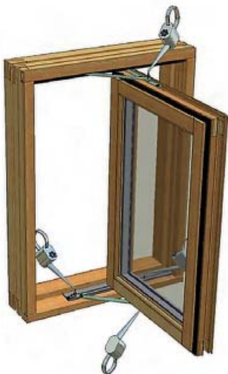
Figure 7.2. Lubricating side projecting gearing
