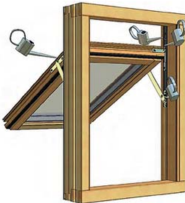
Figure 7.5. Lubricating a top guided gearing
