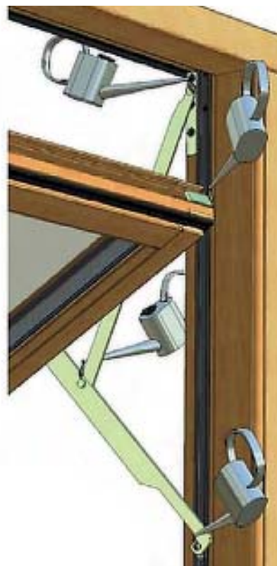
Figure 7.7. Lubricating a top swing gearing
