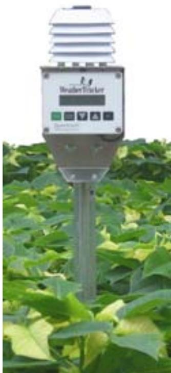
Figure 1: Weather Tracker mounted on 1" conduit
