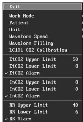
Fig. 14-1 CO<sub>2</sub> Setup Menu
