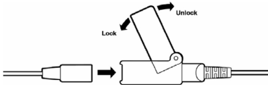
9) Plug the Interface Cable into the SpO2 connector on the side panel of the monitor. Push the cable in until you hear an audible “click”.
