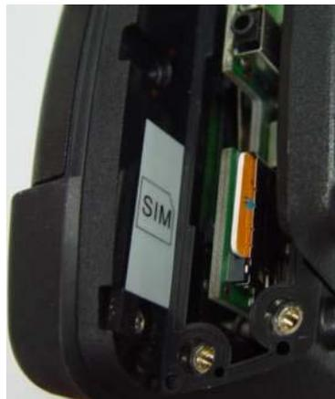
Figure 6-2 Insert SIM card
