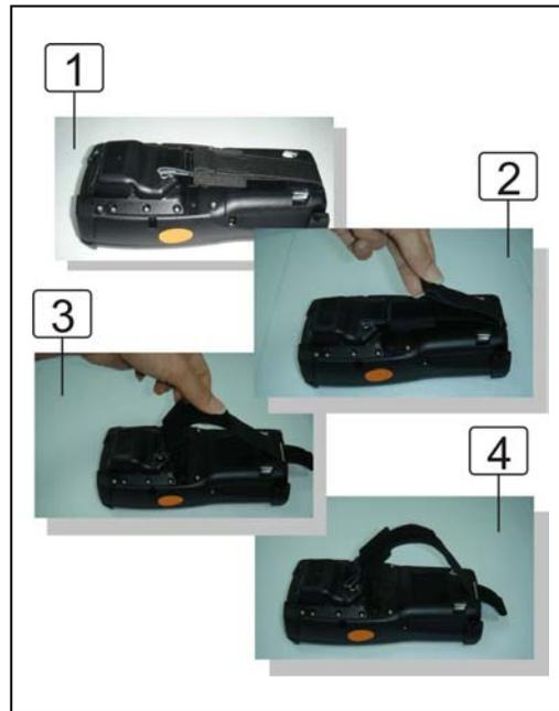
Figure 2-7 Release the Hand strap from PDT
