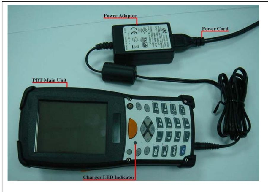
Figure 2-11 Charging with power adapter (PHL-7100 shown)
