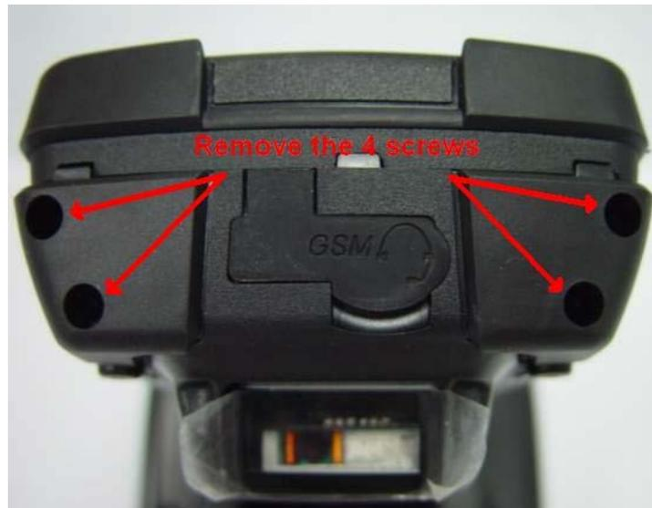
Figure 6-1 Remove screws from End Cap
