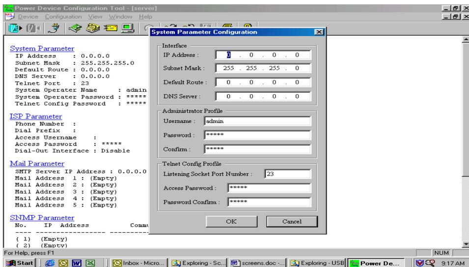
22. This is the System Parameter Configuration screen fill in all the information: the IP Address (required), the Subnet Mask, the Default Route (Gateway) and the DNS Server. Use the Tab key to move from one field to the next field. Then click OK.
