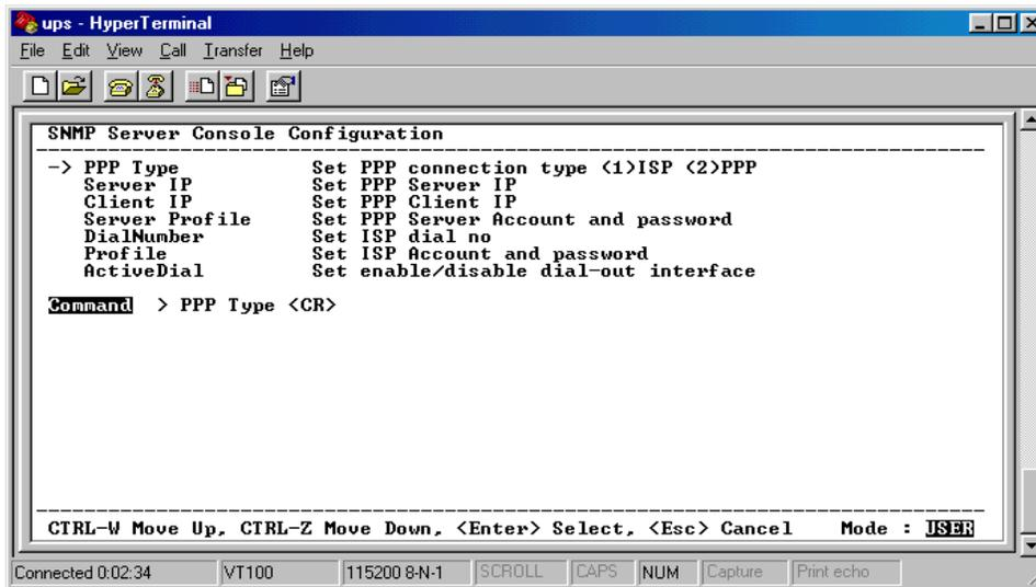
16. Enter in the PPP Type, Server IP, Client IP, Server Profile, Dial number, the ISP account/password and the enable/disable dial-out interface (not required). Hit the “Escape” key to return to the main menu.
