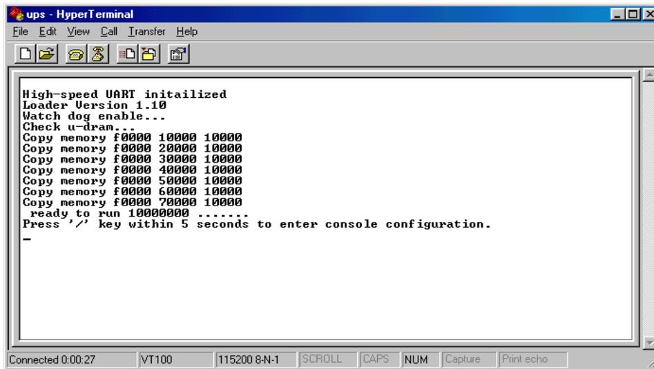
12. When the message “Press ‘/’ key within 5 seconds to enter console configuration” appears press the forward slash key (/) within the 5 seconds or the CIC will time out and then you have to start over.
