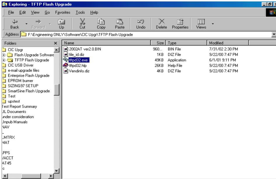
1. Create a folder (TFTP Software Upgrade). Copy the following files to the folder: 2002AT ver2.0.BIN (example), file\_id.diz, tftp32.exe, tftp32.hlp, and Vendinfo.diz. The first file **.BIN** is the actual Software upgrade file, which is available for downloading from our web site. The last four files are on a 3.5" floppy disk included with the CIC package.
