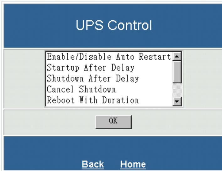
19. This screen allows the User to Control the shutdown and restarting of the UPS. The UPS Control screen, list the commands that can be executed manually. Then click OK.
