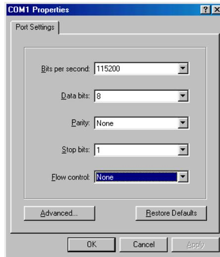
8. Configure the port settings. Bits per second: "115200", Data bits: "8", Parity: "None", Stop bits: "1", Flow control: "None". Click OK.
