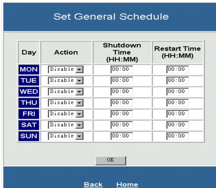
20. This screen allows the User to schedule daily shutdowns and restarts of the UPS. Then click OK. The Computer Interface Card (CIC) will NOT issue the shutdown command to the connected UPS during AC Fail, UPS Battery Low, and UPS Fault conditions. It only notifies users or system administrator of the event. Network node management software like HP OpenView will need to be customized with certain thresholds whether or not to shutdown the Operating System.
