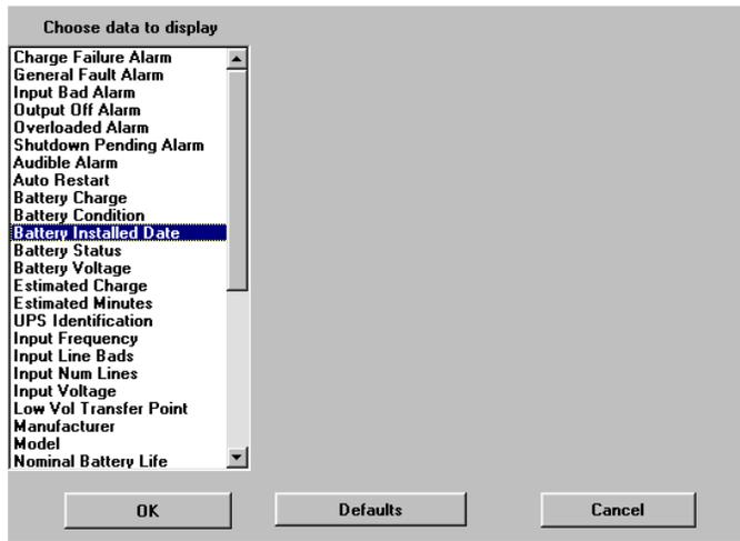
23. On the left hand side of the View Graphic screen, there are seven fields that display data. The user can change any one of these fields, to display the data that they choose, by clicking on one of the fields. Then this screen will appear. Once the selection has been made, click OK.
