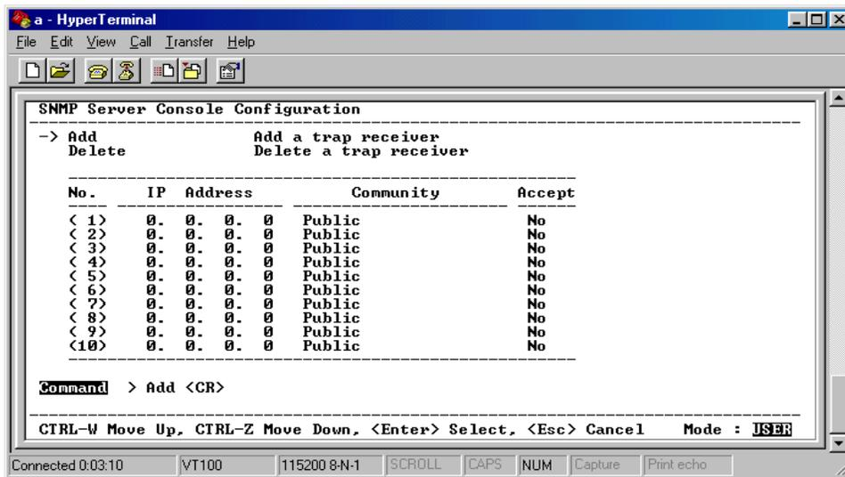
18. Arrow down to Trap and hit enter. This screen allows the user to send Traps about the UPS to ten IP Addresses (not required). Also, you may determine the severity levels and what type of access, read only or read and write, to assign to a particular IP manager. Hit the "Escape" key to return to the main menu.
