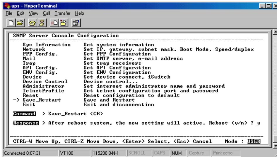
20. After rebooting the system, the new settings will be activated. Reboot (y/n)? Hit the “y” key then hit enter. Once the system has rebooted, cursor down to Exit then hit enter.
