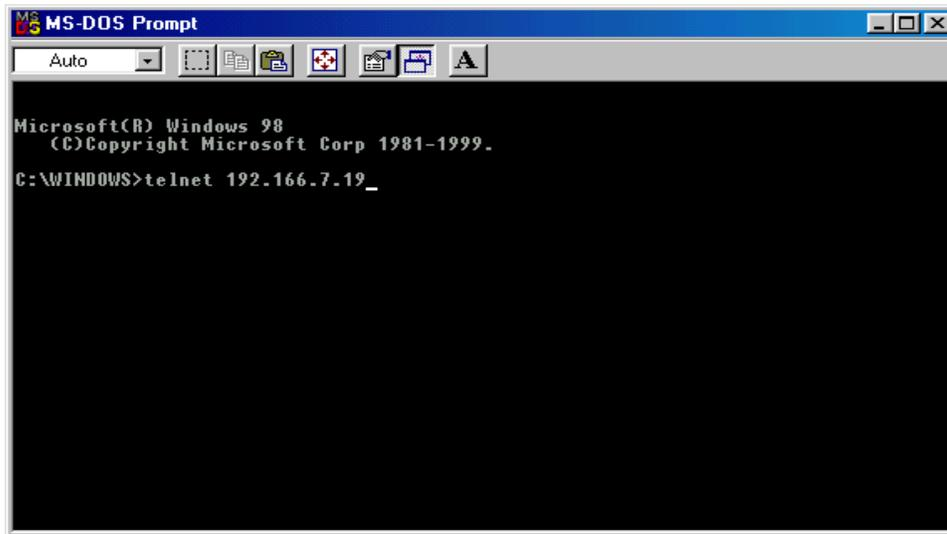
2. This is an example. At the MS-DOS Prompt type telnet 192.166.7.19 (IP Address). Then hit enter.
