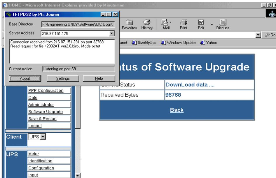
5. The TFTP Server is Flash Upgrading the CIC to the new version of Software. The Software Upgrade takes approximately thirty-five minutes to complete.
