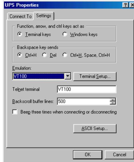
10. Open the Settings Tab. Function, arrow and ctrl keys act as: Terminal Keys, Backspace key sends: Ctrl+H, Emulation: VT100, Telnet terminal: VT100, Backscroll buffer lines: 500. Click OK.
