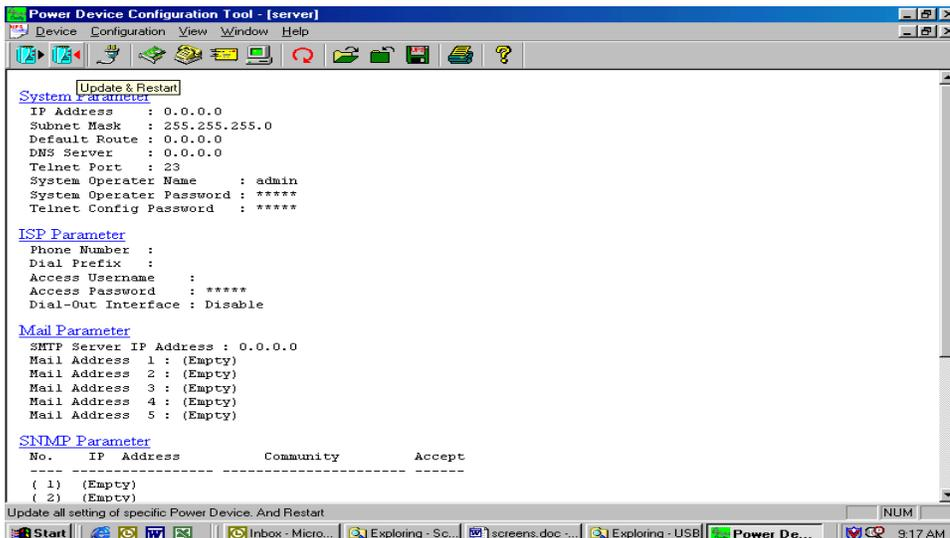
23. This is the Power Device Configuration Tool screen. After you have entered in all of the pertinent information, you have to **Update and Restart** to save all the information that was entered into the System Parameter Configuration screen. The Update and Restart icon (with the red arrow) is right beneath the “Device” drop down menu.
