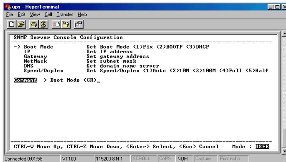
15. Pick IP, then hit enter. Enter in the IP Address (required), the Gateway Address, the Subnet Mask and the DNS. Hit the "Escape" key to return to the main menu.
