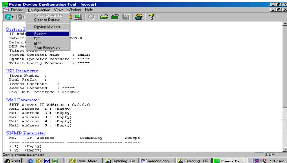
21. This is the Power Device Configuration Tool screen. On the Toolbar open Configuration. Then open System.
