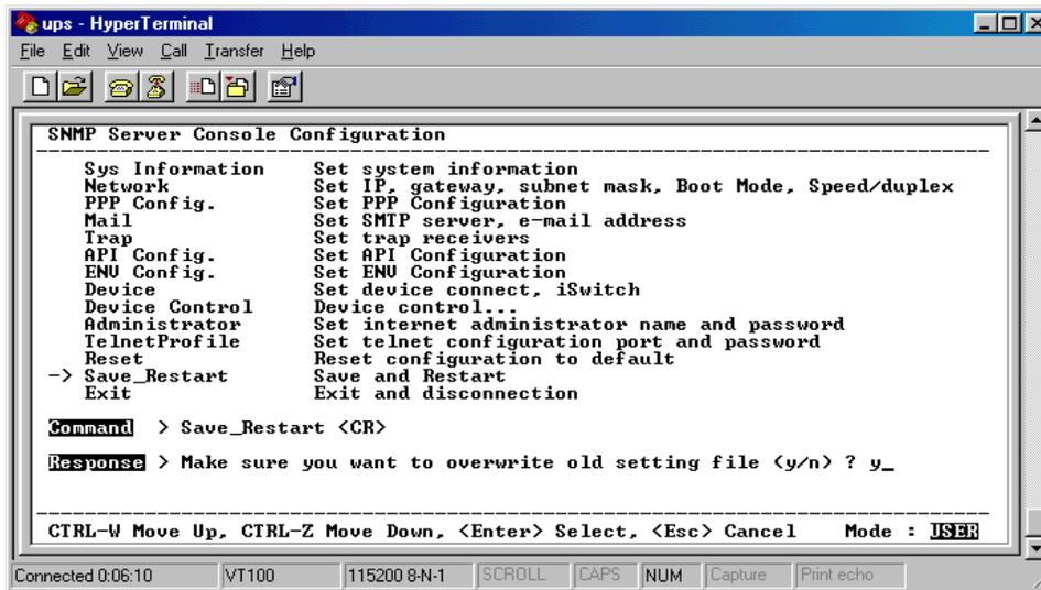
19. Once you have finished with the entire configuration, cursor down to Save\_Restart and hit enter. Make sure you want to overwrite the old settings (y/n)? Hit the "y" key, then hit enter.
