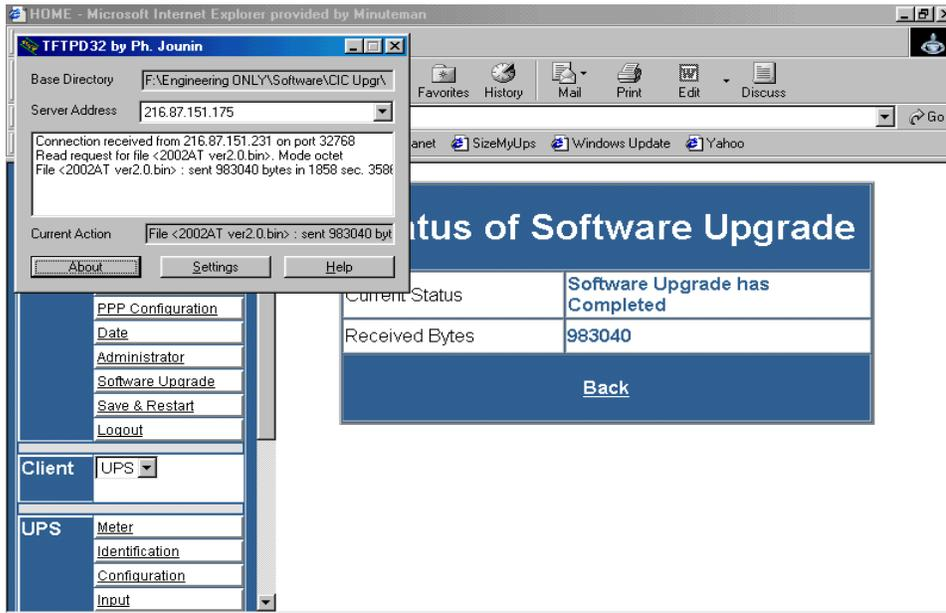
6. The transferring of the Software Upgrade file is complete. Close the tftp32.exe program. Open **“Save & Restart”**. The **“Save & Restart”** function must be performed to save all of the changes. The CIC is ready for normal operation.
