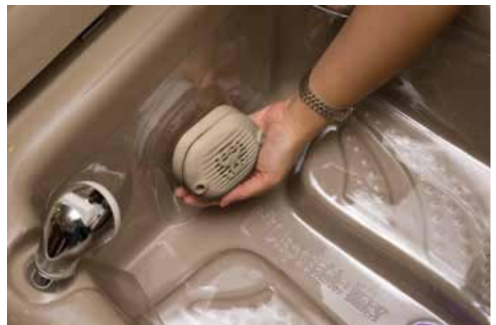
2. Cradle SaniSmart™ wet-end in your palm. Do not hold with your thumb. Jet will attach itself to dry-end. Adjust to align accordingly.
