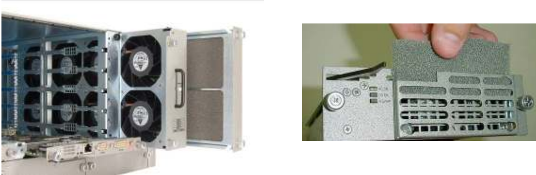
Figure 19 – Shelf Air filter and Power supply air filter extraction
