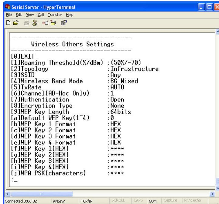
Fig 54. Wireless: Open authorization and none encryption
