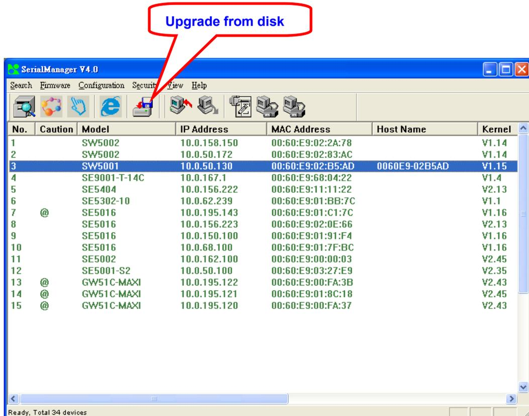
The user can enter the window for downloading by firstly clicking a designated network device, and then selecting the submenu option **Upgrade from disk** in the main menu option **Firmware**, or directly clicking the button **Upgrade from disk**. And then the user can select and download the required firmware from the disk, as shown in the figure below:
