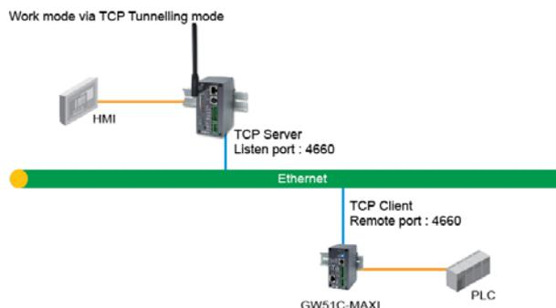
Fig 9. TCP Tunneling Mode
