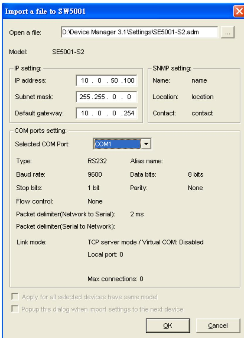
The user can also select several devices at one time, and lead the parameter information of a standard parameter file into all the selected devices by selecting **Apply for all selected devices have same model**.
