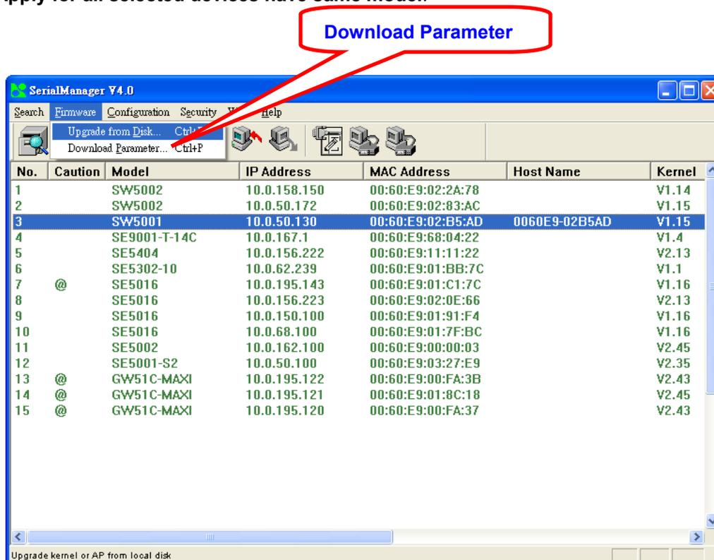
In addition for some devices with JFFS2 file system supported, the user can download the related parameter data into the device that supports the JFFS2 file system through a submenu **Download Parameter**. See details as the figure below:
