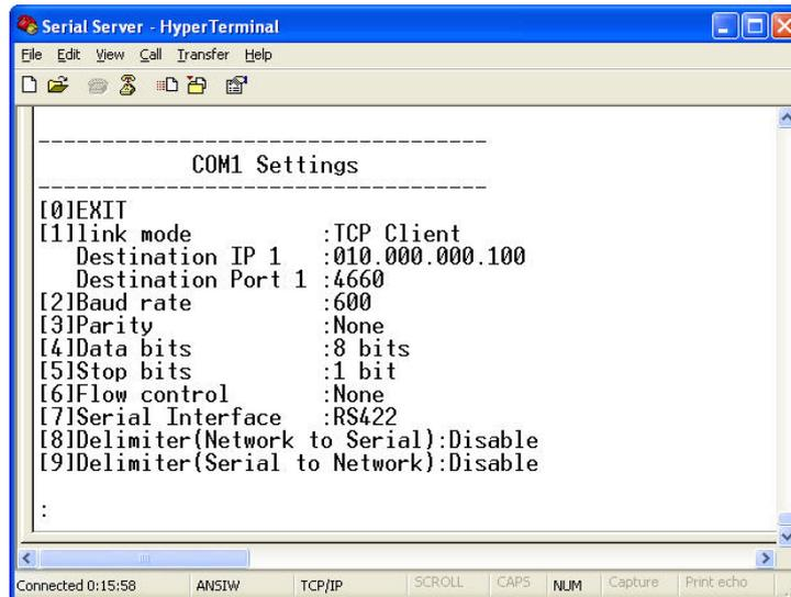
Fig 60. TCP Client mode in link mode
