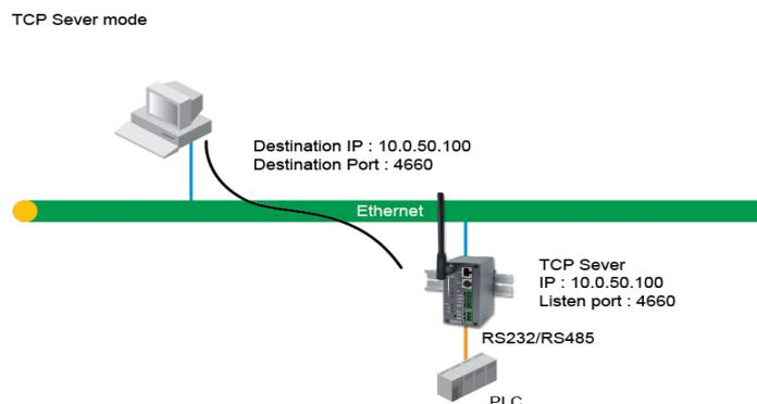
Fig 6. TCP Server in Virtual COM Mode
