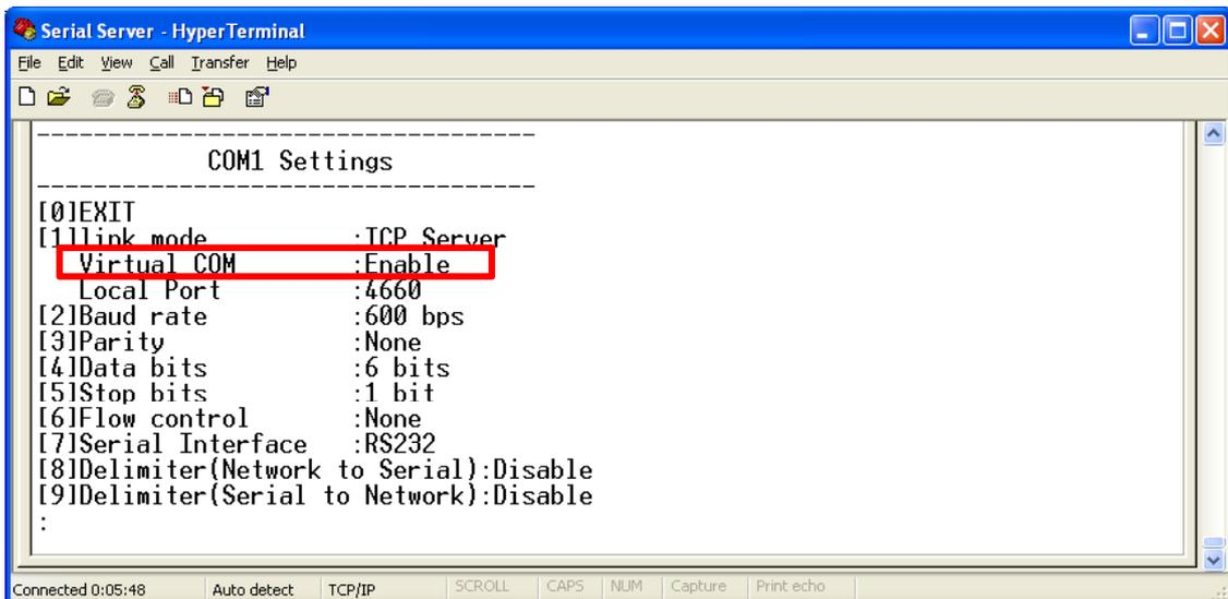
Fig 70. Enable Virtual COM mode by Telnet
