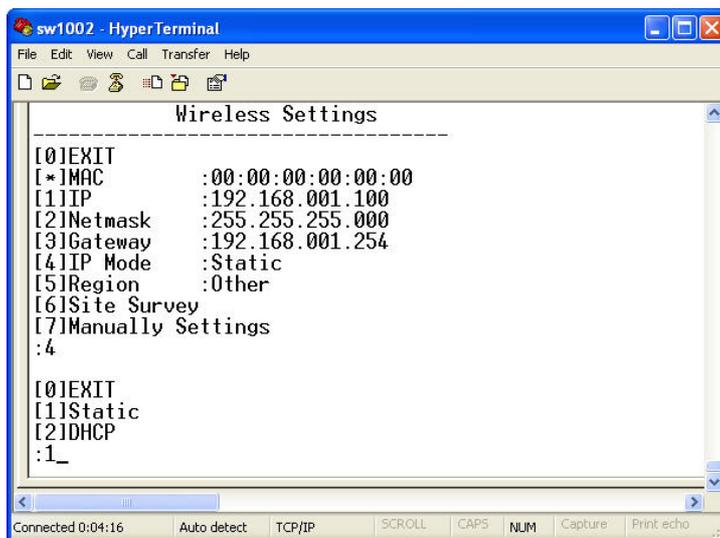
Fig 47. Configure Wireless IP mode by Telnet
