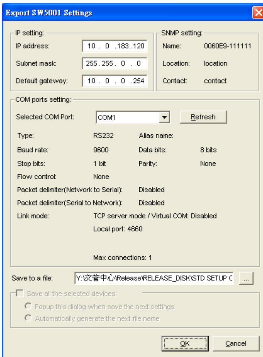
The user can also select several devices at one time, and save the parameter information of these selected devices into a designated parameter file by selecting "Save all the selected devices".
