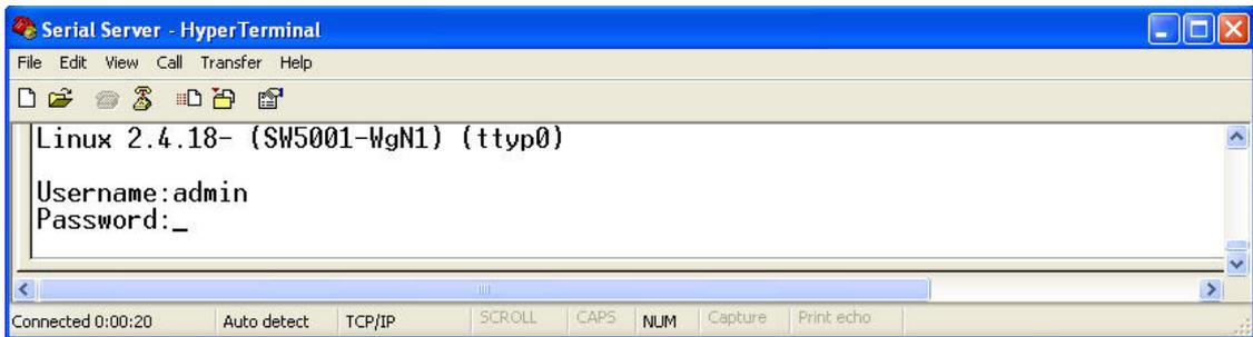
Fig 69. Login into SW5001 by Telnet or Console
