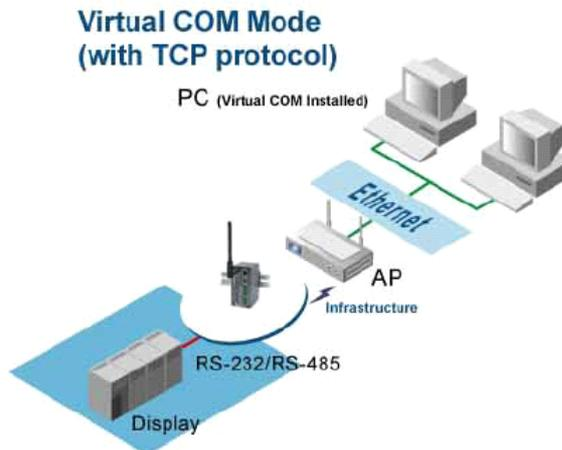
Fig 5. TCP Connection in Virtual COM Mode
