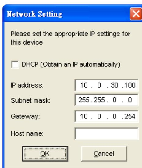
Fig 2. IP settings for SerialManager Utility tool
