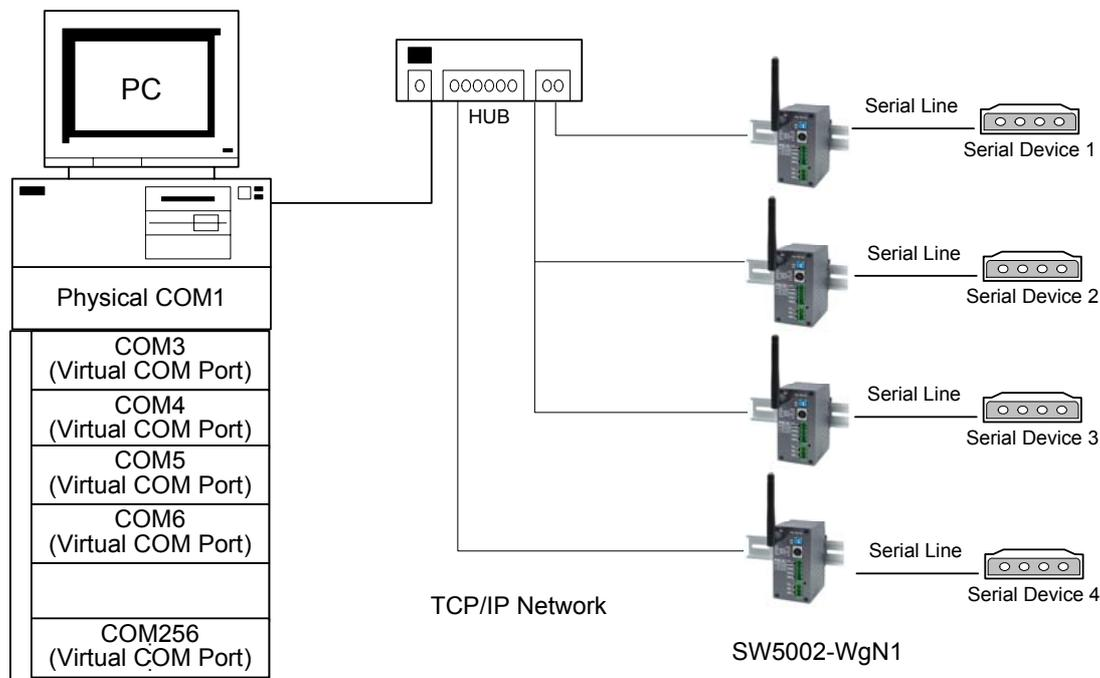
Fig 67. Setup of a Virtual COM driver
