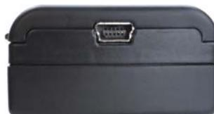
At the back there is a mini USB connector, which is used for charging and data transfer. The SD card is preloaded with the Nanoconfig program, which is used for uploading flight declaration and changing the settings of the NANO. Flight declarations can be also uploaded using a serial interface cable or Bluetooth (See chapter 5.1 for more details).
