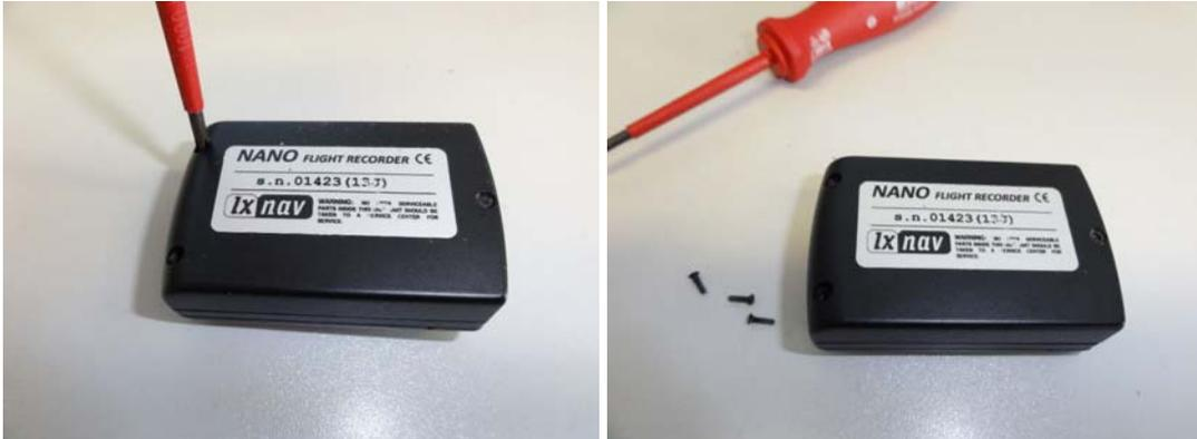
Open the cover and remove the battery.
