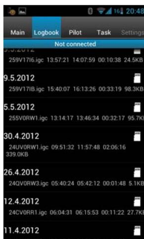
After the downloading of logbook data is finished, a short press on the desired flight will start the download process. If the flight size is big, the download may take more than minute. Flights are downloaded into NanoConfig folder. With a long press on the flight the downloaded flight can be shared with other applications installed on your smart phone (Gmail, SeeYou (not available), OLC (not available) , Google Docs, Facebook).
