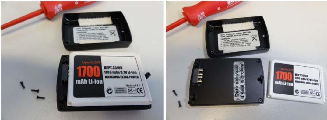
Insert a new Nokia 3310 battery (Li-Ion). Make sure that the contacts are properly aligned. Close the cover and screw back three screws gently.
