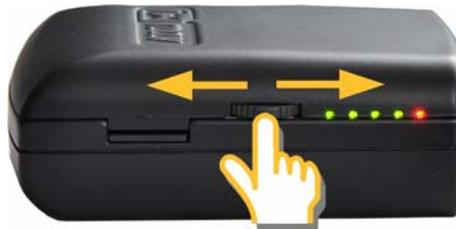
Press it and NANO flight recorder will power on. Press or move the rocker button for a long time and the NANO flight recorder will switch off. When flying press or move the button for a short time and a pilot initiated event will be recorded and the flight recorder will then log 30 fixes with a recording rate of one second.
