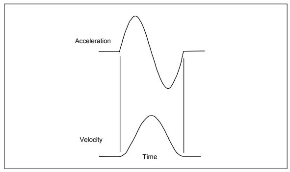
FIGURE 1-4 SHORT MOVE COSINE VELOCITY PROFILE
