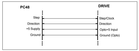
FIGURE 4-2 CONNECTION TO STEP DRIVES
