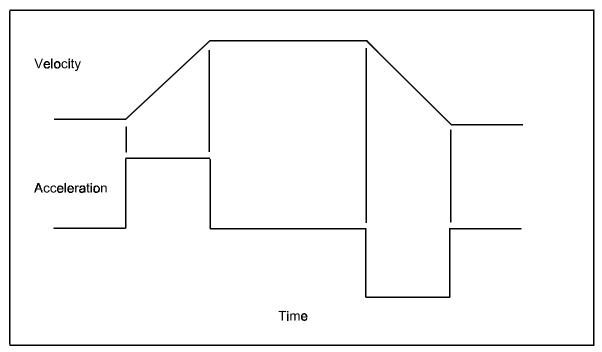
FIGURE 1-1 TYPICAL VELOCITY PROFILE
