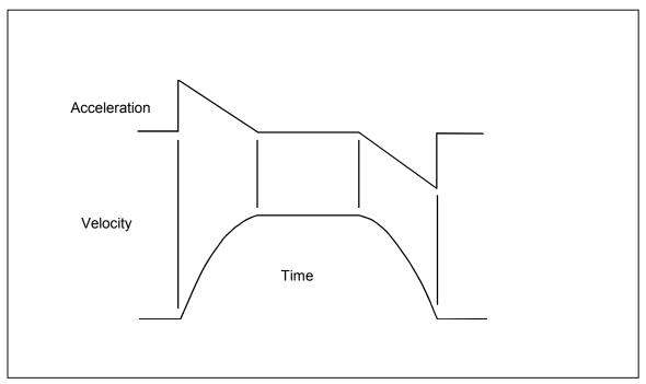
FIGURE 1-2 PARABOLIC VELOCITY PROFILE
