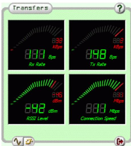
The green numbers shows a current value, the red numbers shows a max received value. A red line specifies a max value in the last five seconds.
