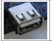
**USB Host Port:** Uses CH376T Host interface chip. Enables connection of USB mass-storage as well as human interface devices to FleaFPGA. USB 2.0 full-speed compatible. CH376T can be accessed from the FPGA side via 1.) CH376T UART TX and RX pins connected to pins #107 and #89 on the FPGA respectively or 2.) Through a dedicated SPI channel. Please refer to Appendix B as well as the CH376T device datasheet for further details.
