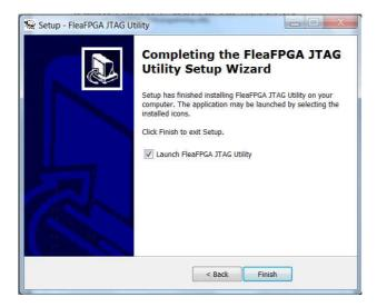
iv. Make sure the 'Launch FleaFPGA JTAG Utility' option is ticked and then click finish. FleaFPGA utility will now run and request the path of "ddtcmd.exe". This file can typically be found in the following path (assuming you've installed the 64-bit version of lattice Diamond here): C:\lscc\diamond\2.2\_x64\bin\nt64
