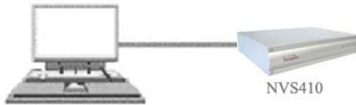
Figure 3-2. Direct connection using crossover LAN cable
