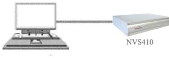
Figure 3-4. Direct connection using crossover LAN
