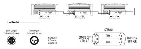
For installations where the DMX cable has to run a long distance or is in an electrically noisy environment, such as in a discotheque, it is recommended to use a DMX terminator. This helps in preventing corruption of the digital control signal by electrical noise. The DMX terminator is simply an XLR plug with a 120  $\Omega$  resistor connected between pins 2 and 3,which is then plugged into the output XLR socket of the last fixture in the chain. Please see illustrations below.
