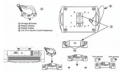
Regardless of the rigging option you choose for your LED X-men, always be sure to secure your fixture with a safety cable. The fixture provides a built-in rigging point for a safety cable on the hanging bracket as illustrated above. Be sure to only use the designated rigging point for the safety cable and never secure a safety cable to a carrying handle.
