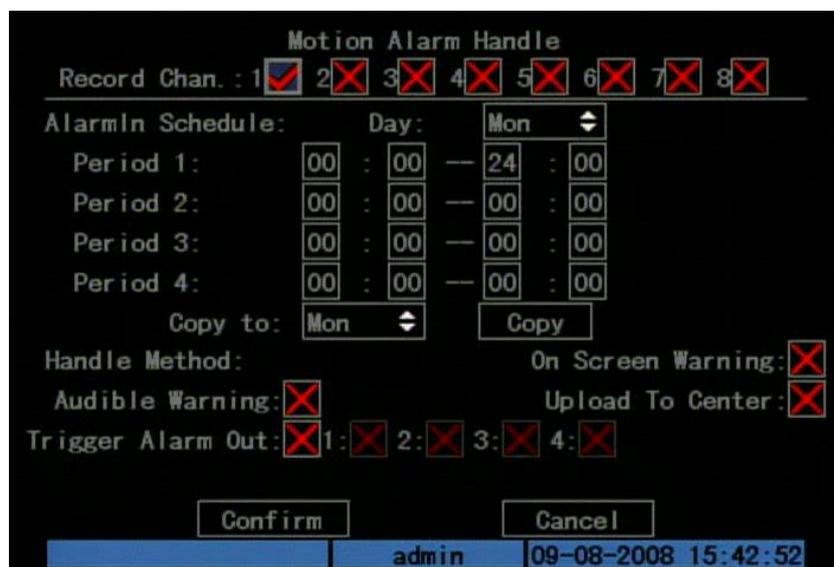
Fig. 5.19 Motion alarm handle setup
