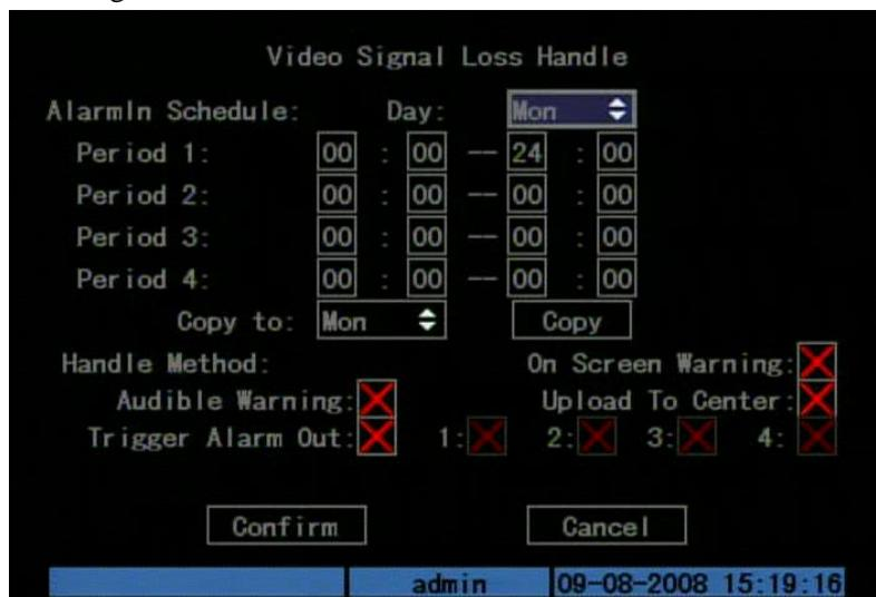
Fig. 5.17 Video signal loss handle setup
