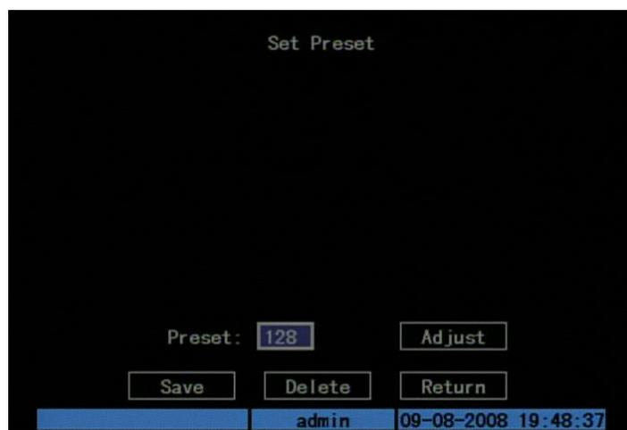
Fig. 5.32 PTZ preset setup
