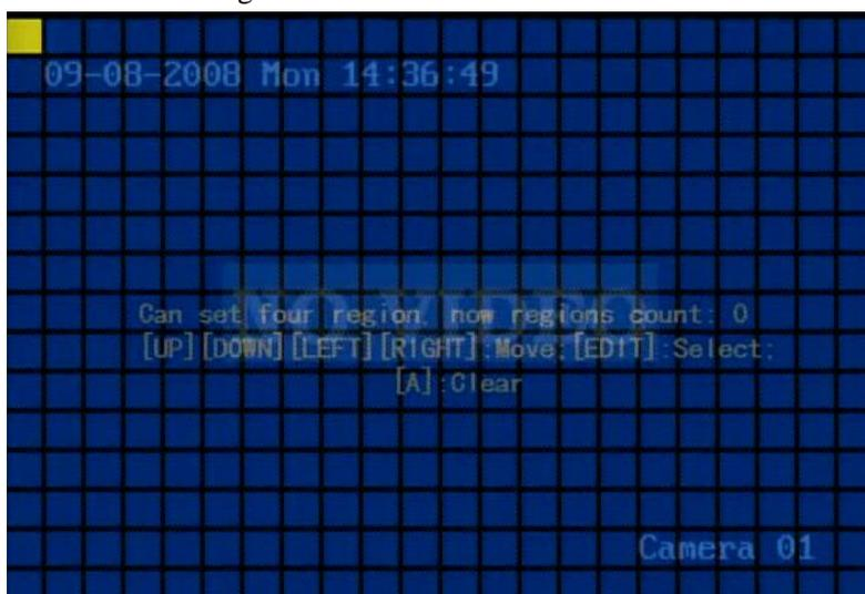
Fig. 5.14 Mask area setup
