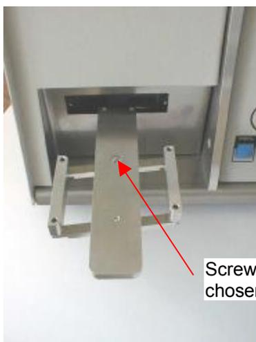
Screw fixing the chosen width
