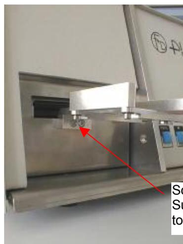
Screws fixing the Supporting table to the printer
