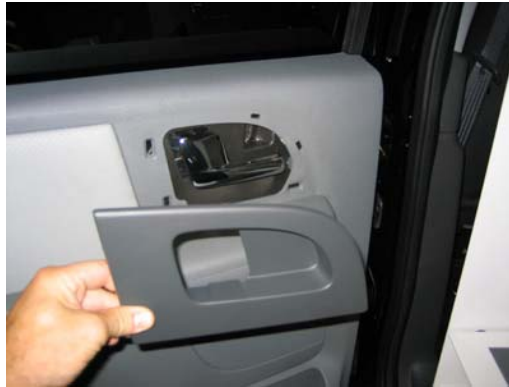
Remove plastic trim piece. Metal clips hold on trim
