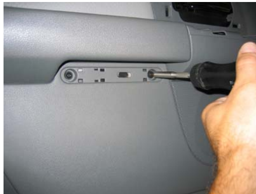
Remove trim piece covering torx screws under door panel armrest and remove screws
