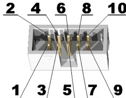
**TDI** Input **Test Data In**. This is the serial data input for the shift register.
