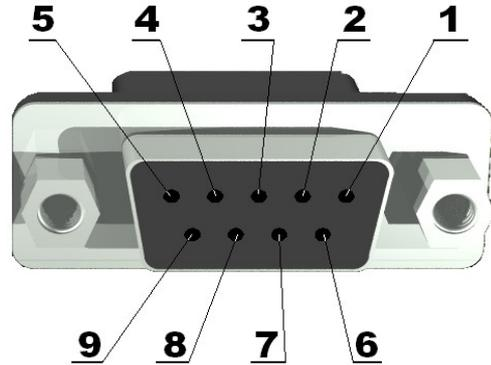
**TXD0** Output **Transmit Data**. This is the asynchronous serial data output (RS232) for the shift register on the UART controller.
