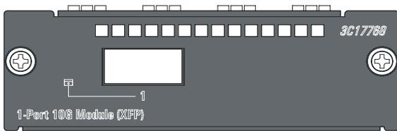
This module provides one 10 Gbps XFP optical interface. You can select the following XFP transceivers as required. A one-port 10 GE XFP interface module provides one 10 Gbps XFP optical port. You can insert an XFP transceiver into the port to connect it to another XFP port through an optical fiber. You can select the XFP transceivers list in [Table 1-18](#) as required.
