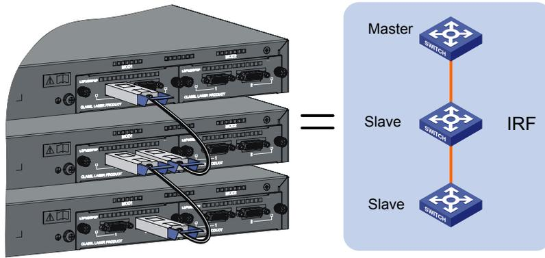
**Figure 3-27** The ring connection mode
