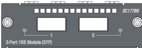
A dual-port 10 GE XFP interface module provides two 10 Gbps XFP optical ports. You can insert an XFP transceiver into the port to connect it to another XFP port through an optical fiber. You can select the following XFP transceivers in [Table 1-18](#) as required.
