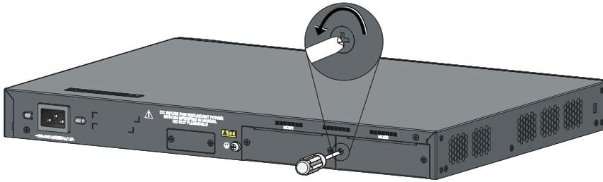
**Step3** Hold the fastening screws on the front panel of the XFP interface module, and gently push the interface module in along the slot guide rail until the interface module is in close contact with the switch.
