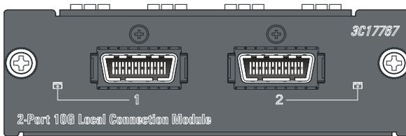
A short-haul dual-port 10 GE CX4 interface module provides two 10 Gbps electrical ports and supports CX4 electrical and protocol standards. Only 3Com's CX4 power cables can be used for connecting the CX4 ports. A CX4 cable is hot swappable and its maximum transmission distance is 3 m (9.84 ft.), which is suitable for short-distance connections only.
