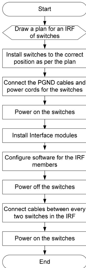
**Table 3-4** Description of the installation flow for an IRF of switches
