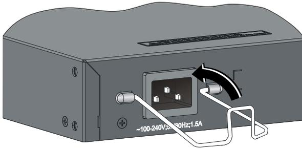
**Figure 3-17** Connect an AC power cord to a horizontal AC power socket (2)
