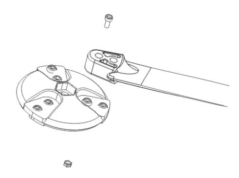
• Attach the Rotor assembly (hub and blades) onto the generator shaft and torque nut (shaft) securely with included Allen wrench without exerting undue force (~22ft-lbs.)
