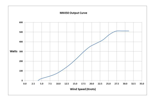
The electricity generated by the MarineKinetix MK450 is converted from 3-phase AC to 12 volt DC power by the Micro-computer Controller. This DC power can be used to operate 12 volt appliances directly, charge 12V batteries, or operate AC appliances with the use of an AC Inverter (not supplied). A 24 volt model is also available.
