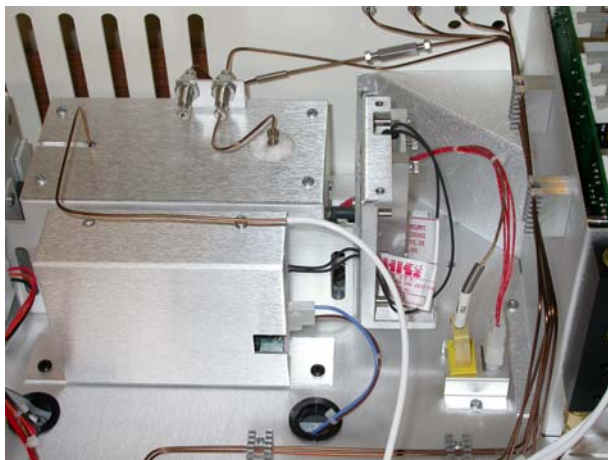
Figure 9. RCP Detector Showing Column Outlet and Standby Fittings
