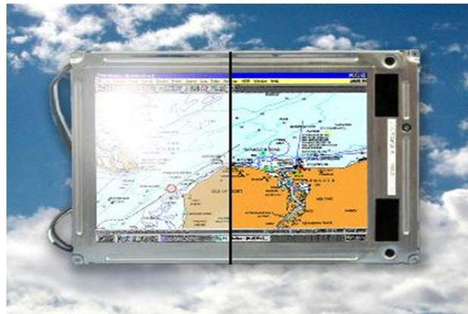
Figure 4 – Comparison with and without Optical Bonding
