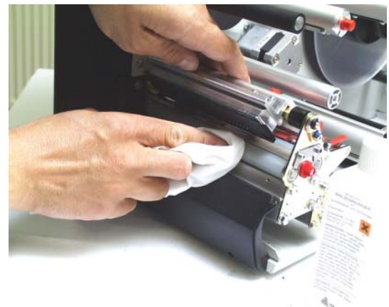
Fig. 4 Rotate the printhead upwards before cleaning it.
