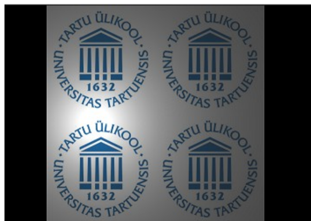
Illustration 57: Image of the UT logo UV mapped to a quad in a way it repeats two times in both directions.
