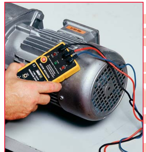
Phase & Motor Rotation Tester Model PMR-1 verifying motor rotation.
