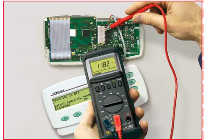
Digital Multimeter Model CA5220 measuring voltage levels on an alarm touch pad.
