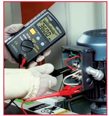
The Digital/Analog Megohmmeter Model 1026 quickly verifies the isolation of all the connections in the box.
