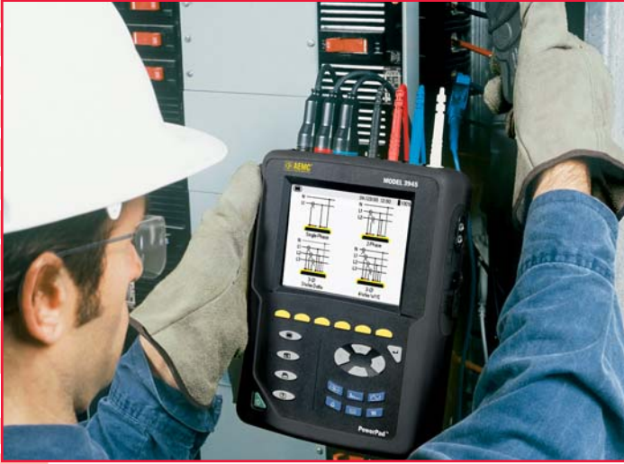
The hand strap on the side of the PowerPad™ Model 3945 allows one hand free to conduct the testing.
