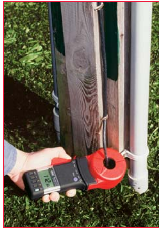
Model 3731 performing a ground rod resistance check.
