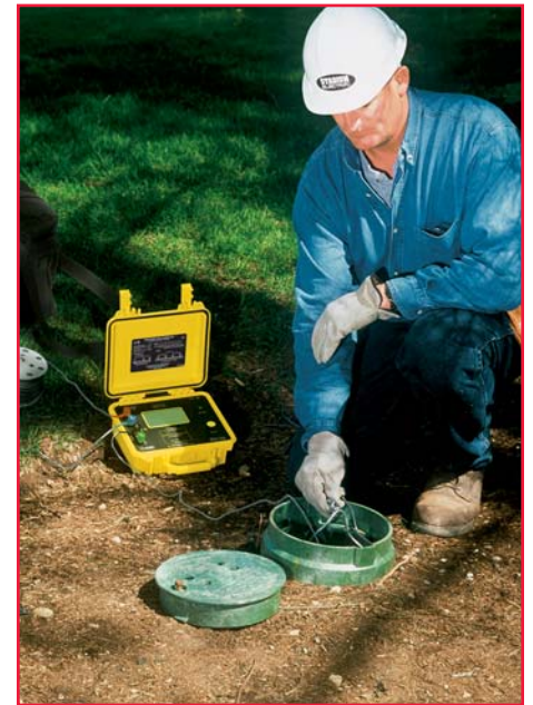
Digital Ground Resistance Tester Model 4630 performing a 3-Point ground resistance test on an individual rod.
