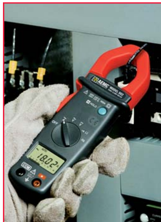
Clamp-On Meter Model 502 monitoring phase current on a power panel.
