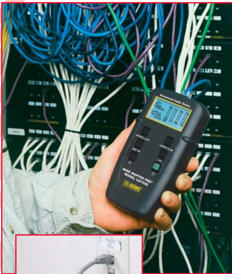
LAN and Cable Tester Model CA7028 used to locate and test a cable from the patch panel to an office a few hundred feet away.
