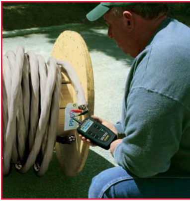
Cable Tester Model CA7024 is used to check length of a power cable on a reel.
