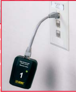
LAN and Cable Tester Model CA7028 used to locate and test a cable from the patch panel to an office a few hundred feet away.
