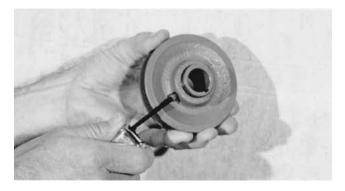
Adjust motor pulley to its closed position for maximum fan speed or increments of 1/2 turn open (maximum of 5 turns open) for reduced fan speed. Tighten set screw on flat area only.
