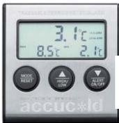
Every unit is equipped with a Traceable Thermometer/Alarm that simultaneously displays minimum, maximum and current interior temperatures and provides a visual and audible signal when the temperature inside the unit falls outside the set temperature range.
