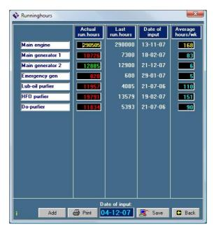
Enter the running hours, (which you can find on the dial of the equipment/engine), in the box 'Actual running hours', then it turns yellow. "Save" the running hours, then the box turns green.
