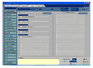
Marad starts automatically with the maintenance module. Then the result of the program, the working list/ week list, will be showed. The week list tells you what to do that week according to the established maintenance system. You also can take a look forward in the maintenance. The week list can be printed with the button Print, right below.
