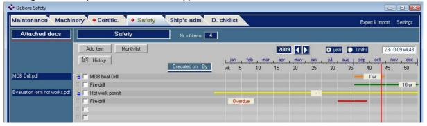
The vertical red line indicates the actual date. The length of the horizontal coloured lines indicate the length of the interval of an item. The colours of the lines indicate the status of the items.
