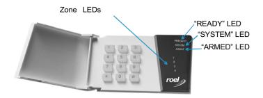
The keypad is the device which helps program the system, enter data and display system state.
