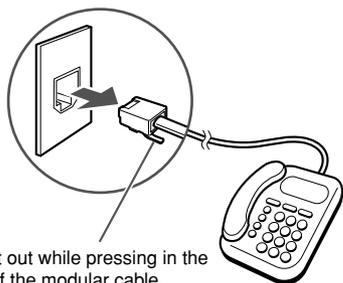
Pull it out while pressing in the clip of the modular cable.
