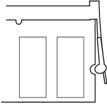
In this case, further push the memory into the slot.
