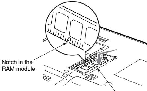
**6 Attach the expansion RAM module slot cover as it was.**
