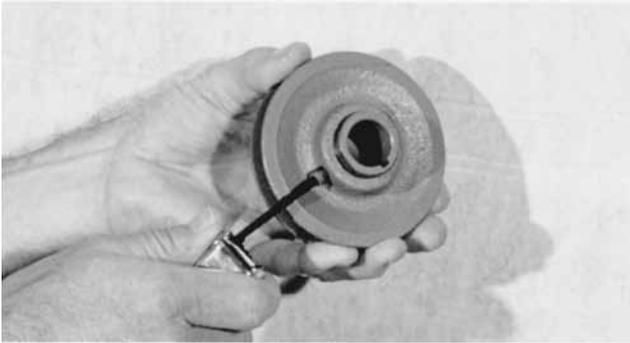
1. Adjust motor pulley to its closed position for maximum fan speed or increments of 1/2 turn open (maximum of 5 turns open) for reduced fan speed. Tighten set screw on flat area only.
