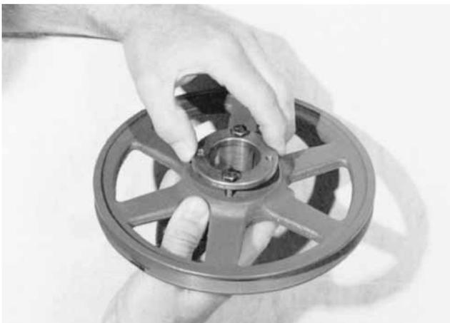
3. If supplied, install taperlock bushing into shaft pulley.
