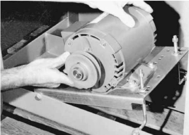
2. Install motor pulley to the motor shaft and install motor to the motor plate. Pre-punched holes are provided for most common motor frame sizes.
