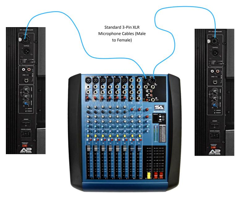
This example shows how to connect two MainShock speakers to a standard Mixer. This application requires (2) XLR 3 pin male to female cables. Seismic Audio offers these cables. The model number is: SAXLX-25.
