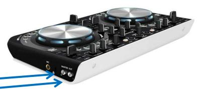
Use the Seismic Audio cable: SAXFRM-2x5 to plug your DJ Controller or any other RCA output device into the XLR inputs of the MainShock speakers.
