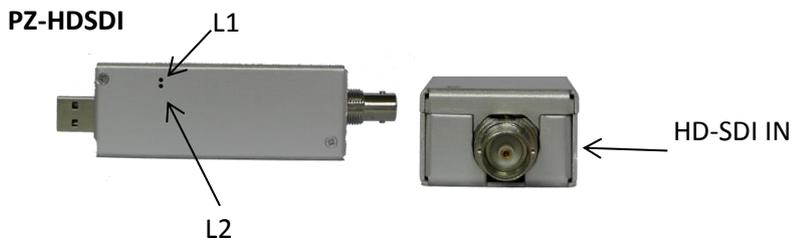
L1 & L2 Flashing Indicates no input signal detected
