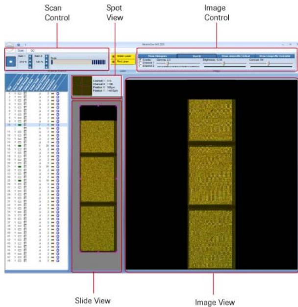
Figure 7: Example of a Run Time Window
