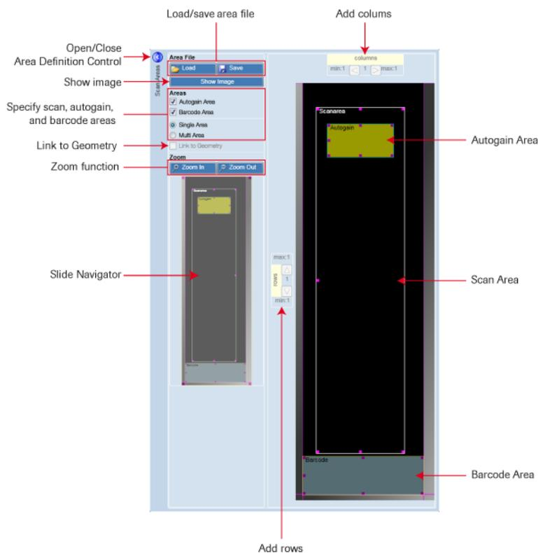
**Figure 5: Components of the Area Definition Control**
