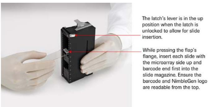
Figure 1: Inserting Slides into the Slide Magazine
