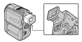
You turn the LCD panel over and move it back to your camcorder body with the LCD screen facing out. You can operate with the touch panel using the viewfinder in CAMERA or MEMORY mode (p. 63).
