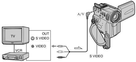
Connect the yellow plug of the A/V connecting cable to the video jack on the VCR or the TV.
