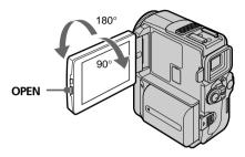
When closing the LCD panel, set it vertically, and swing it into the camcorder body.
