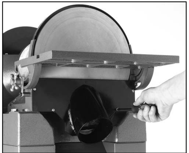
Figure 12. Attaching dust port.
