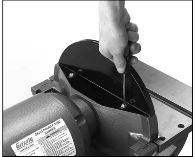
Figure 11. Attaching disc guard.
