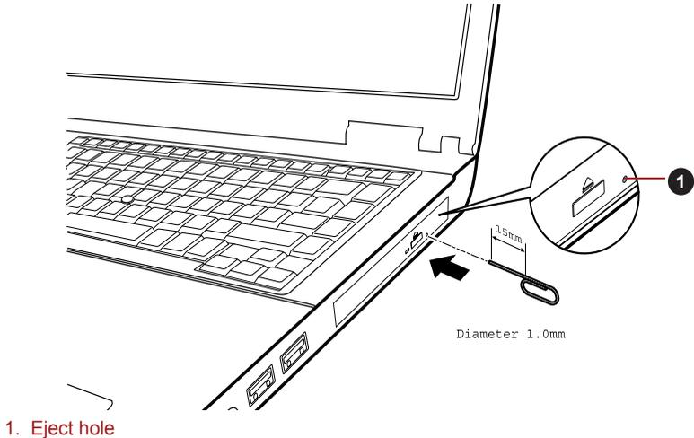
Figure 4-9 Manual release with the eject hole
