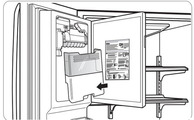
4. Avoid touching the ice-detecting sensor when replacing the ice bin. See the label on the ice compartment door for details.
