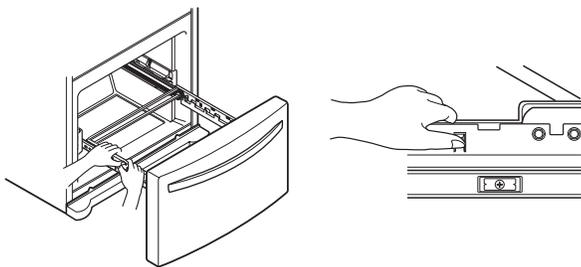
Remove the screws ② of the rail on both sides.
