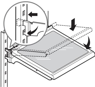
**⚠ CAUTION:** Make sure that shelves are level from one side to the other. Failure to do so may result in the shelf falling or spilling food.
