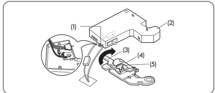
1. Open the door. Remove the top hinge cover screw (1). Lift up the cover (2).
