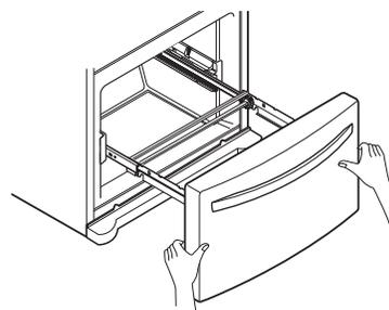
With both hands, hold the center bar and push it in to allow both rails to slide in simultaneously.
