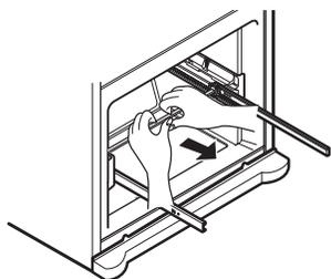
Hook the door support into the rail tabs on both sides.
