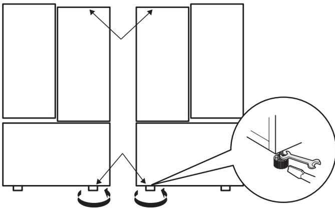
**NOTE:** Having someone push backward against the top of the refrigerator takes some weight off of the leveling legs. This makes it easier to adjust the legs.
