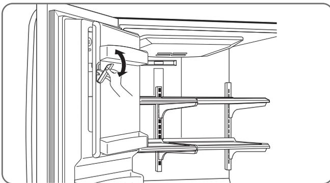
2. To remove the in-door ice bin, grip the front handle, slightly lift the lower part, and slowly pull out the bin as shown.
