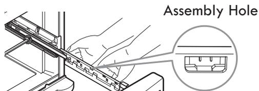
**NOTE:** Make sure that the left and right rail covers are attached to the correct rails. See picture below.
