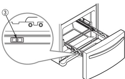
Align the tabs on the covers with the assembly holes on each rail and snap the rail covers in place to secure.
