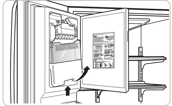
3. To reinstall the in-door ice bin, slightly slant the bin during replacement to avoid contact with the icemaker.
