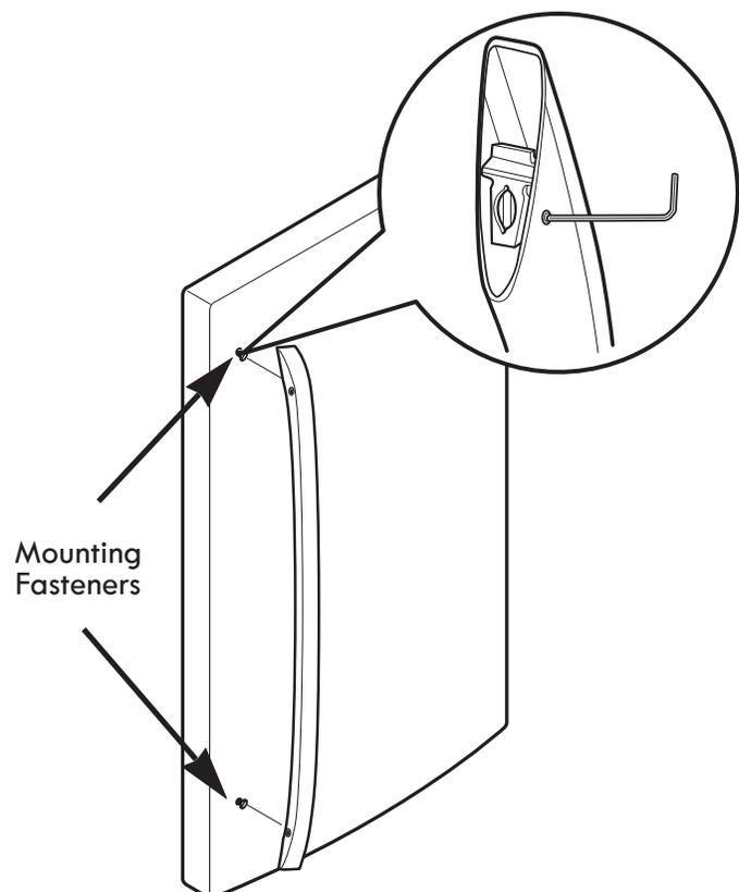
**NOTE:** Removing the doors is always recommended when it is necessary to move the refrigerator through a narrow opening. If it is necessary to remove the handles, follow the directions below.
