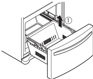
Press the tabs on each of the rail covers and lift them up to separate from the rail assembly.
