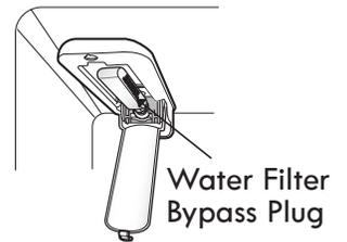
**CAUTION:** DO NOT operate refrigerator without water filter or water filter plug installed.
