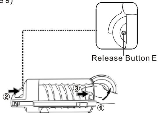
**3** Clean the main filter and prefilter with a soft-bristled brush (not included) and rinse with cold water. Allow both items to dry completely for 24 hours.
