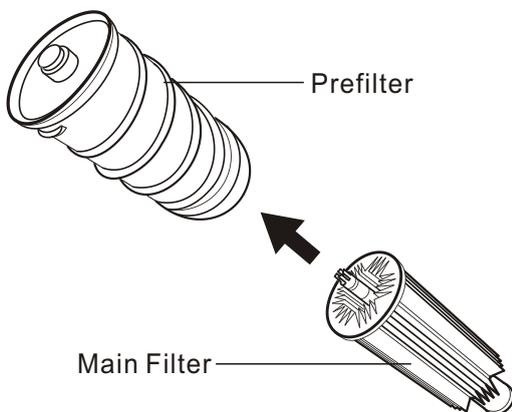
**2** Hold onto the main filter and insert into the dust compartment.
