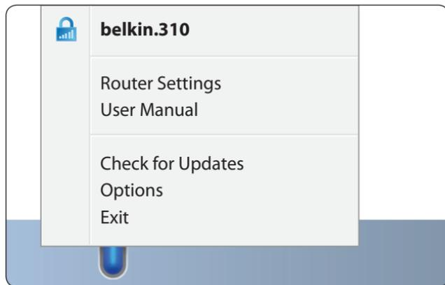
The Belkin Router Manager appears in your system tray (Windows) or menu bar (Mac). Its icon indicates the current status of your Router and also allows you to access your Router's settings to make changes. It also provides quick access to software that came bundled with your Router.
