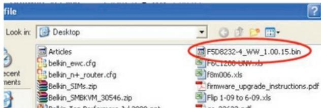
9. Select the firmware file by left-clicking on it and then click the "Open" button in the lower-right corner of the window. This will take you back into the Router's interface.
