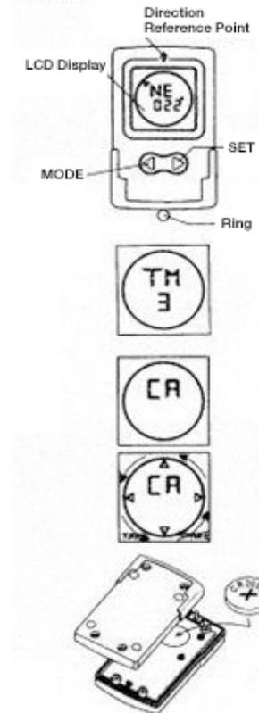
Once calibrated properly, the LCD display will show the direction you are facing while looking through the binocular. The small triangle containing the letter "N" will always point to the north.
