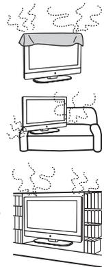
Leave some space around the TV set as shown below. Otherwise, air-circulation may be inadequate and cause overheating, which may cause a fire or damage to the TV set.
