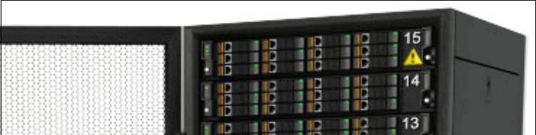
Figure 7-23 Module temperature threshold exceeded
