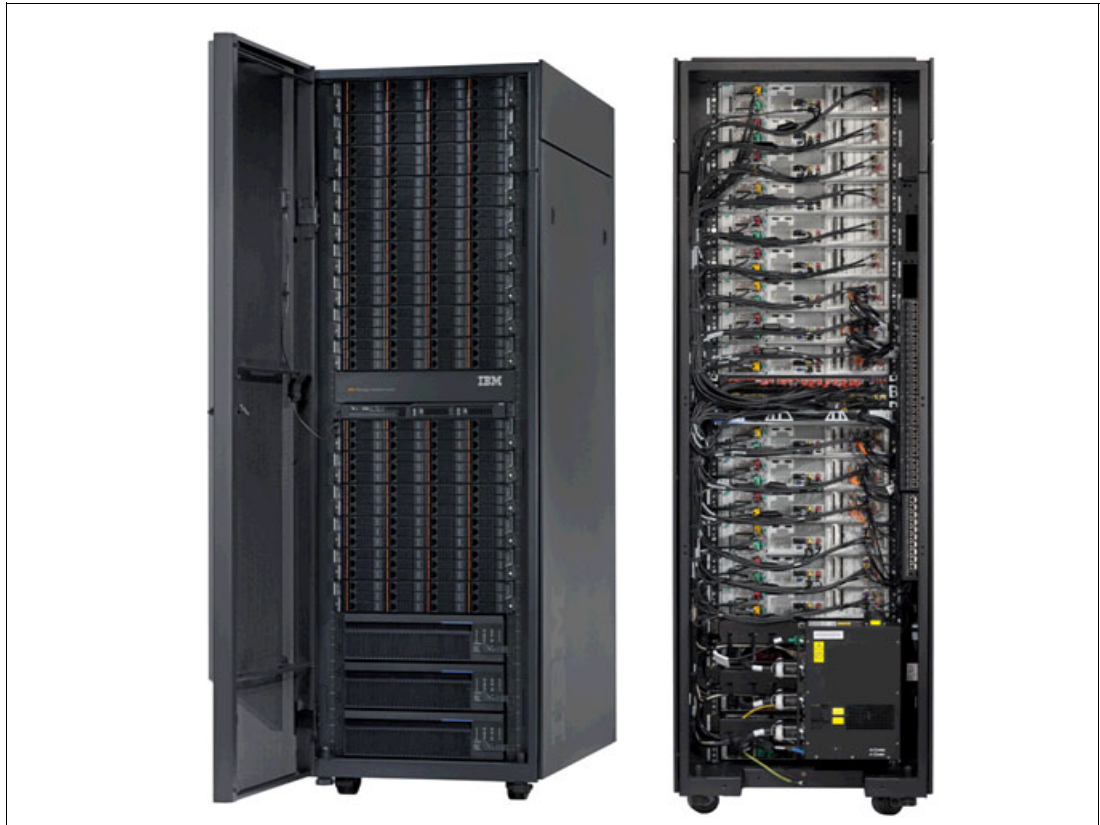
Figure 3-1 IBM XIV Storage System Gen3: Front and rear views
