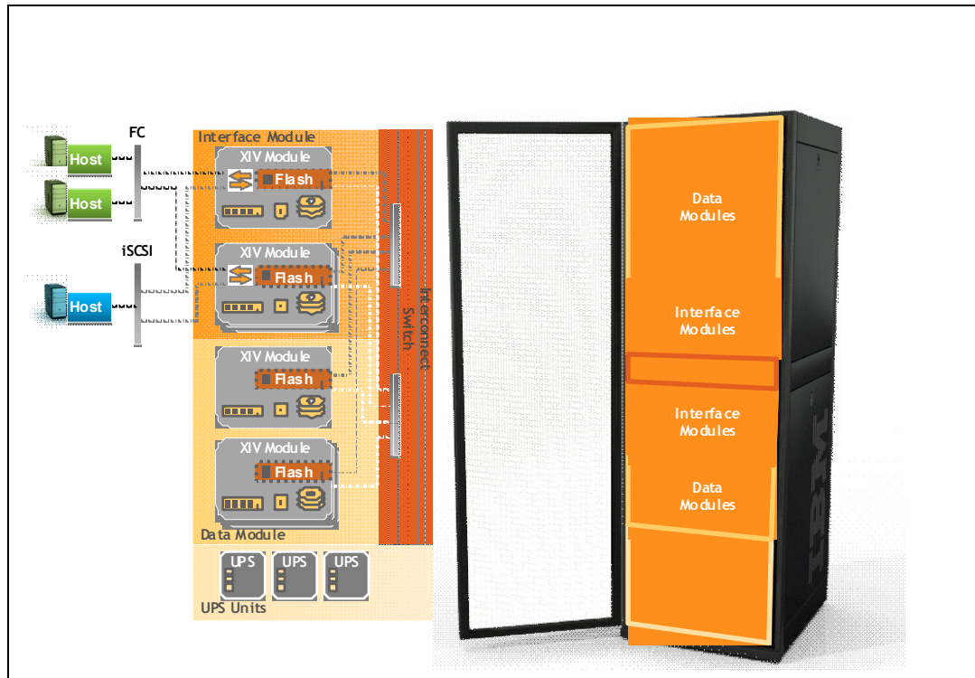
Figure 2-1 XIV Storage System major hardware elements
