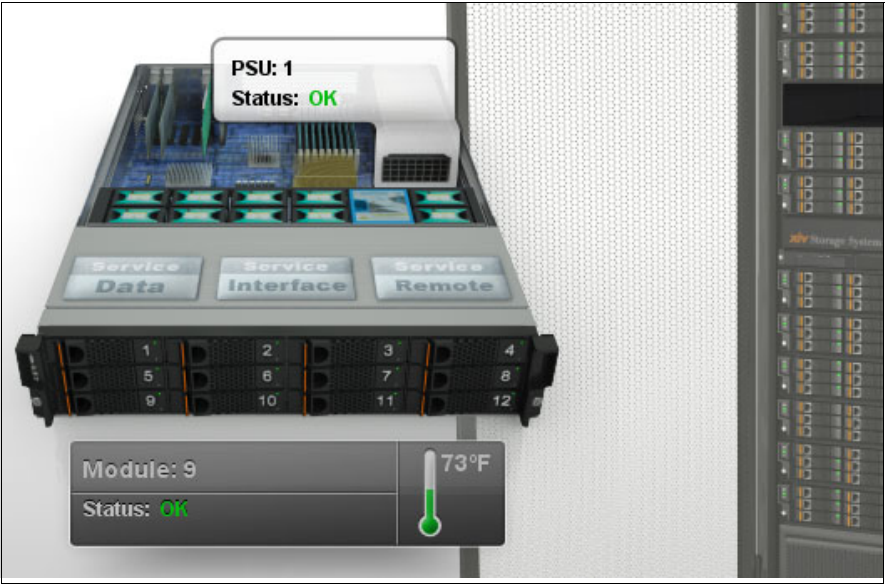
Figure 7-22 Component status in module explosion drawing
