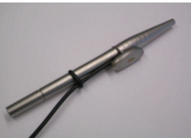
Figure 9: Finger switch mounted on handpiece
