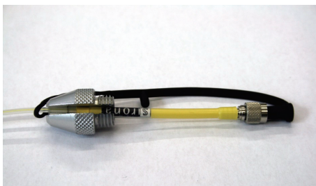
Figure 14: Optical fiber with protection caps
