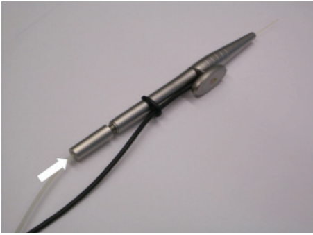
Figure 18: Inserting the optical fiber into the handpiece
