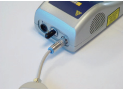
Figure 2: Plugging the Y-connector into the laser unit
