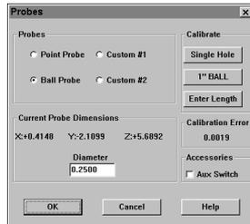
ENTER LENGTH is only used for sheath-type probes that slide over the 1/4" ball probe. See "Enter Tip Length" on page 47.
