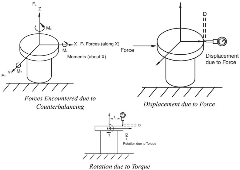
In general, the excessive translation deformations are added directly to the certified accuracy, while the excessive angular deformations of the base affect accuracy as a more complicated trigonometric function of the length of the reach.
