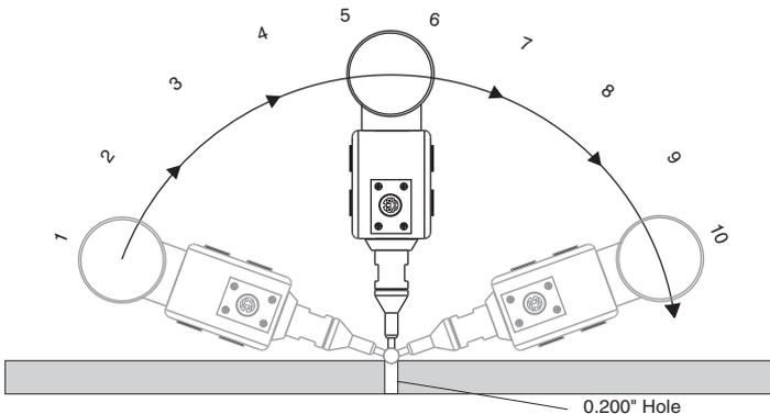
Figure 2-3 Single Hole Calibration
