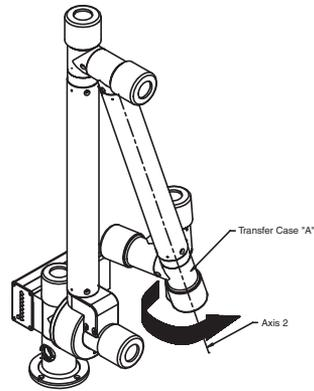
Figure 1-9 Rotate Transfer Case "A" about Axis 2
