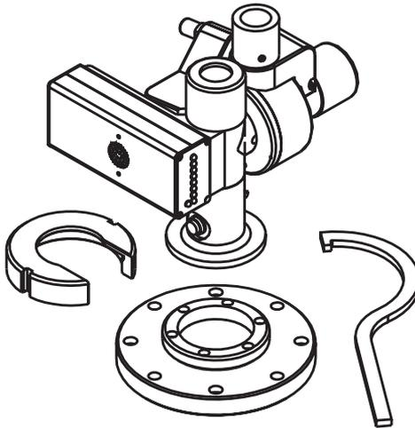
*Figure 1-13 Mounting the Sterling FaroArm*
