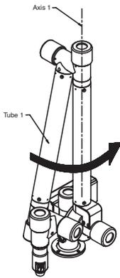
Figure 1-8 Rotate Tube 180 degrees about Axis 1
