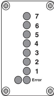
Figure 1-15 Sterling Controller Front View
