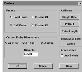
**NOTE:** The probe must be in full contact with the reference sphere for all 27 calibration points digitized. Even one or two poorly digitized points significantly affects the optimization process, which then has an effect on the accuracy of the FaroArm.
