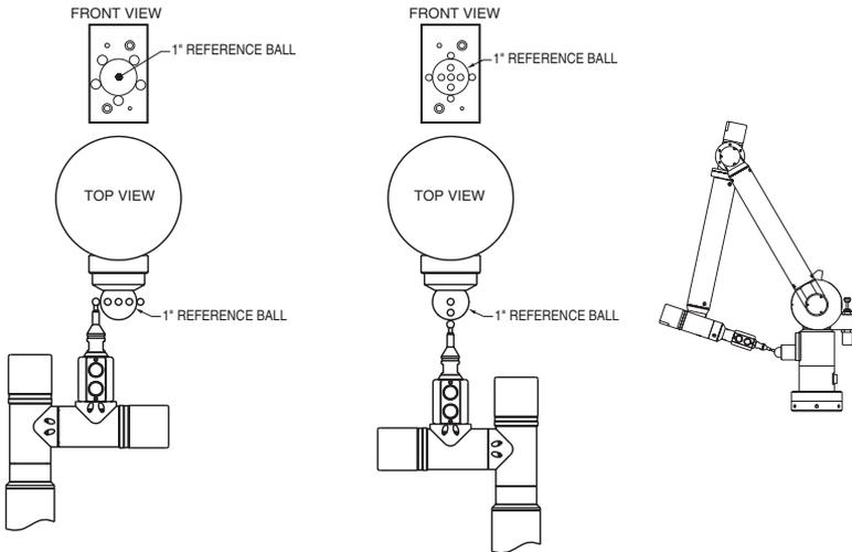
Figure 2-4 1" Reference Sphere Calibration
