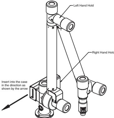
Figure 1-10 Hand Position on FaroArm
