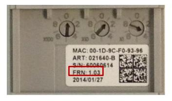
For the communication module, the product nameplate is located under the front cover. The module specific application firmware revision will be in the FRN field.
