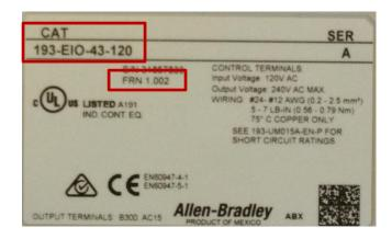
For the control module, the product nameplate is located on the side of the module. The module specific application firmware will be in the FRN field.
