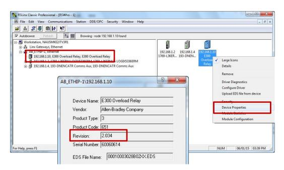
The installed system firmware version number may be determined using RSLinx connected to the overload relay's Ethernet network. Open the RSLinx RSWho dialog and find the E300 Overload Relay. Right click on the desired relay icon and select "Device Properties" from the menu. On the Device Properties dialog, the system firmware revision number will be in the Revision field.
