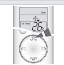
To adjust the temperature, press hutton to set the desired temperature. The temperature can be set between 16°C(61°F) and 30°C(86°F).
