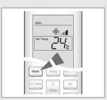
2 To select Auto mode, press Mode button until **Auto** appears on the remote control display.
